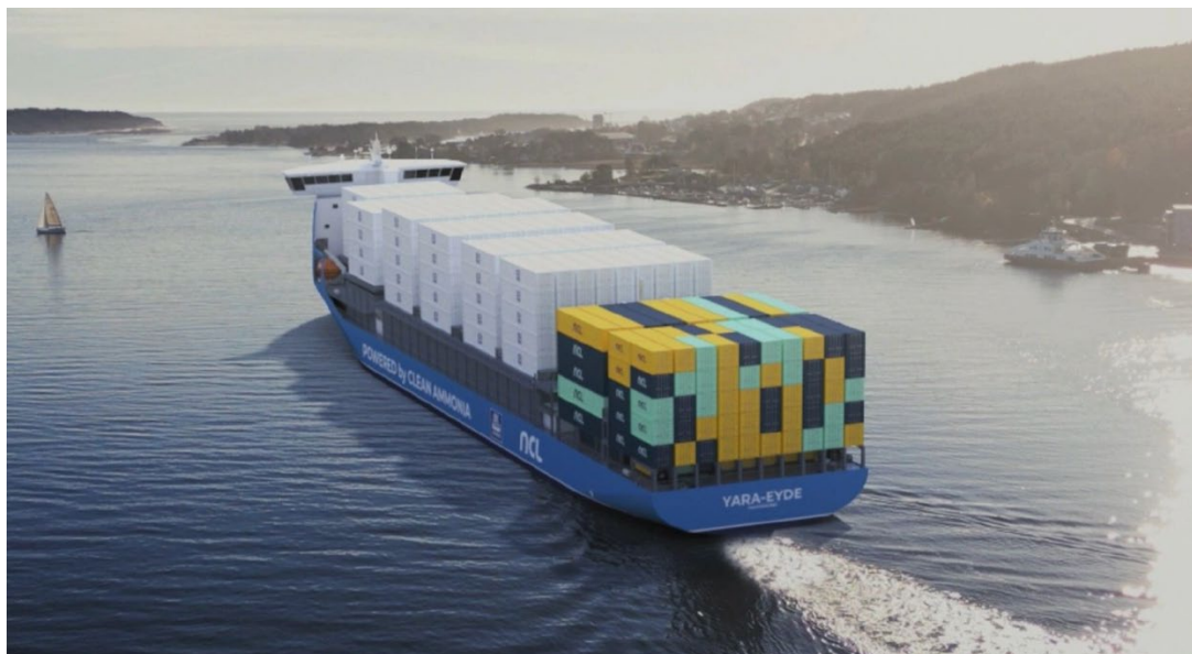
Several zero-emission ideas have been presented, but this is among the more realistic ones: Yara Eide, supposed to be fully operational in 2026 and using green ammonia for its propulsion.
